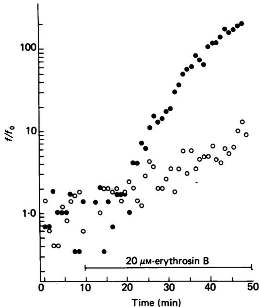
Fig. 1. The m.e.p.p. frequency ( $f$ ) increases with time relative to its initial level ( $f_0$ ) after addition of Erythrosin B ( $20 \mu\text{M}$ ) to normal Ringer solution (O) and calcium-free Ringer solution containing EGTA (●).
