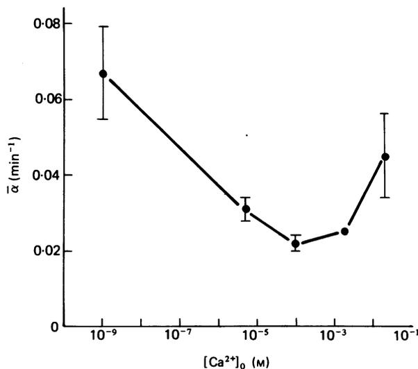
Fig. 3. The mean rate of increase in m.e.p.p. frequency ( $\bar{\alpha}$ ) caused by Erythrosin B ( $20 \mu\text{M}$ ) is a function of the calcium concentration in the Ringer solution ( $[\text{Ca}^{2+}]_0$ ). Calcium-free saline containing 1 mM-EGTA is indicated as  $10^{-9}$  M. Vertical bars indicate  $\pm 1$  s.e. and points represent means of three determinations (six for 1.8 mM-Ca).
